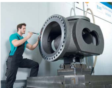
Quality control for the L4NC pump casing
